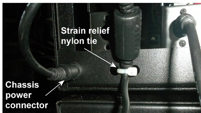
This ensures the fan power cord will not be accidentally pulled out while the blades remain powered.
